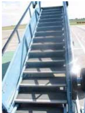
The movable steps are kept outside and are exposed to the weather and a variety of potential contaminants to the walking surface but the profiled rubber treads to the steps still offer reasonable slip resistance.
